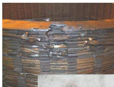
A failed winding where copper sulphide was a factor in the failure
