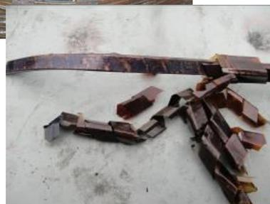
Evidence of copper sulphide from a retired transformer
